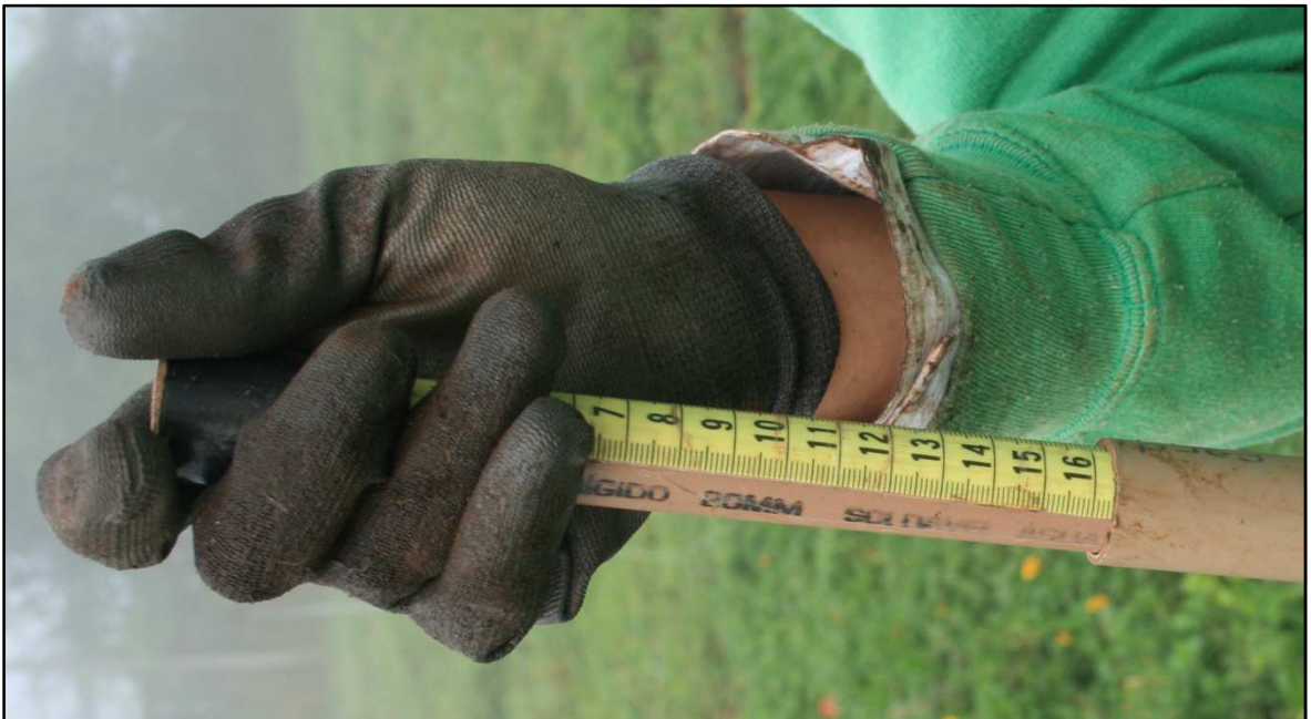
Figura 2. Fita graduada do sward stick
