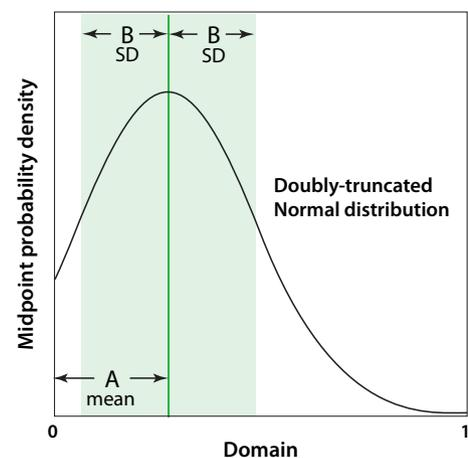
**Figure 2** The midpoint attractor modelled with a doubly truncated Gaussian probability density function with mean  $A$  and standard deviation  $B$ . Parameter  $A$  controls the position of the attractor on the gradient. Parameter  $B$  controls the strength of the attractor (small  $B$  = a strong attractor, large  $B$  = a weak attractor).
